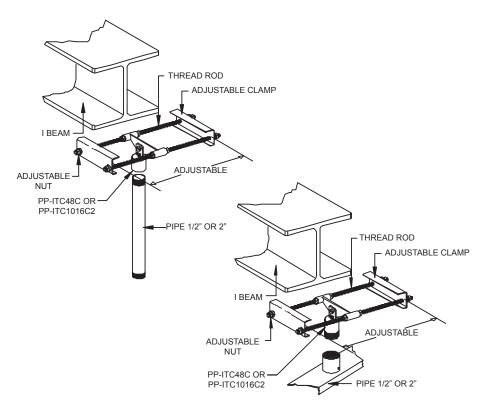
These new clamps can easily support weights up to 175 lbs. (1 1/2") fittings and 350 lbs. (2") fittings properly installed by qualified personnel.
