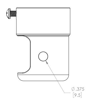
THREAD 1.5" NPT PIPE COUPLER WITH CABLE MANAGEMENT
