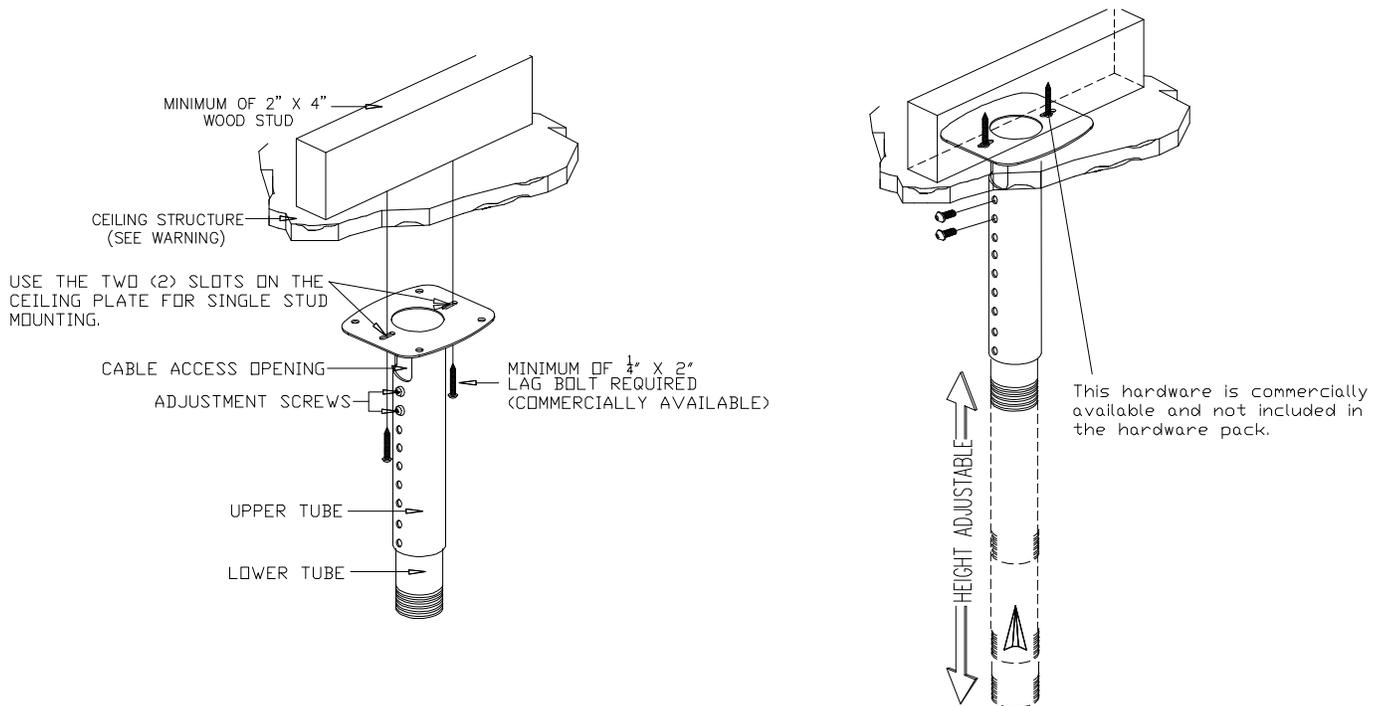
**NOTE:** TO SECURE THE PROJECTOR MOUNT OR MOUNT/ADAPTER TO THE AST-1321, REFER TO THE INSTALLATION INSTRUCTIONS.
