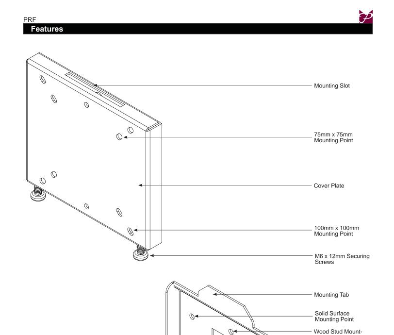
These mounting points also act as mounting points if you decide to mount the PRF to a handibox, using the 6-32 x 1" screws. It is recommended that all electrical wiring be done by a licensed electrician.
