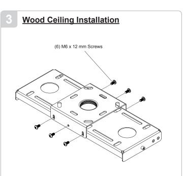
Disassemble the upper and lower base box by removing the six (6) M6 x 12 mm screws. Place the screws aside.
