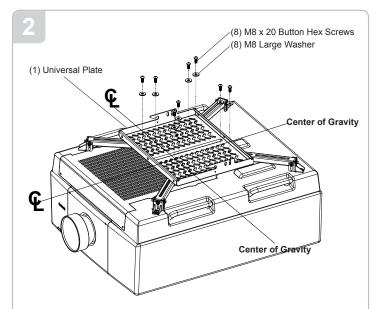
Install the Universal Plate to the Universal Leg Assembly's using eight (8) M8 x 20 Button Hex Screws and eight (8) M8 Large Washers. Tighten the M8 x 20 Button Hex Screws using the supplied M5 Allen Key.
