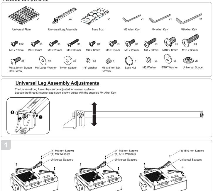
Install four (4) Universal Leg Assembly's using four (4) M6, M8, or M10mm screws depending on projector.
