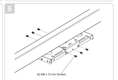
Install the upper and lower base box together by using the six (6) M6 x 12 mm screws disassembled on steps 3.
