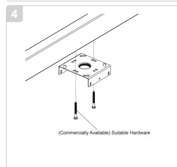
Secure the upper base box using two (2) commercially available hardware.
