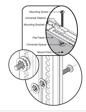
Universal Spacers allow the user to attach the mounting bracket to flat-panels which have recessed or uneven mount points. Each Universal Spacer adds 1/4" to the distance between the mounting bracket and the flat-panel.
