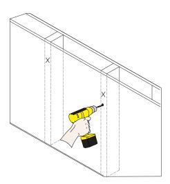
Drill a pilot hole using a M6 or 1/4" drill bit on the stud that was marked on the upper right.
