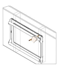
Use a pencil to mark the upper right mounting location of the wall stud.
