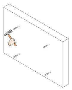
Insert the Finned anchors into each pilot holes. Lightly tap each Finned anchors into place with a hammer.
