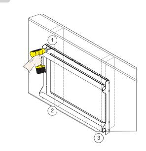
Drill a pilot hole in each of the three (3) marks with a power drill and a M6 or 1/4" drill bit.
