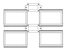
Multiple LMVF mounts can be installed using model specific spacers. Simply repeat step one when installing each of the surrounding LMVF mounts. Use one spacer for each 2x2 installation by mounting it to the wall, or utilize the same spacer as many times needed to complete an unlimited LMVF large matrix video wall.
