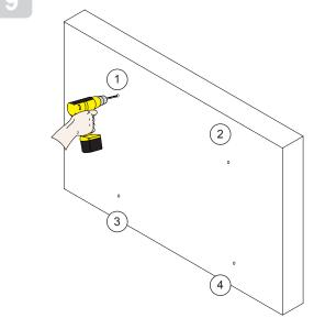
Drill a pilot hole in each of the four (4) mark areas with a 3/8" masonry drill bit.
