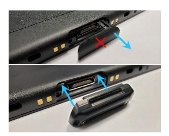
Remove the rubber seal from the bottom of the tablet and discard it. At this point, the tablet is no longer IP65 rated.
