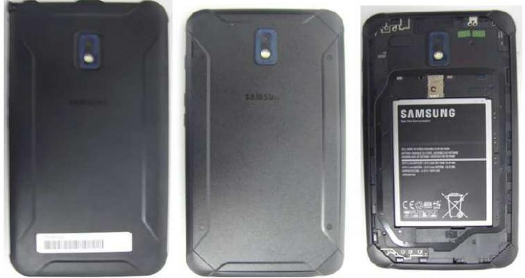
1. Remove the Samsung Tab Active 2 bumper case and back cover. (Figure #1)
