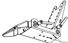
mounting holes for standard Gamber-Johnson motion attachments
