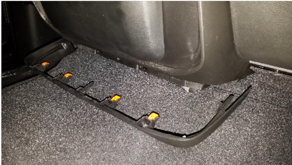
**FIG 1 - Lower Center Panel Removed**
