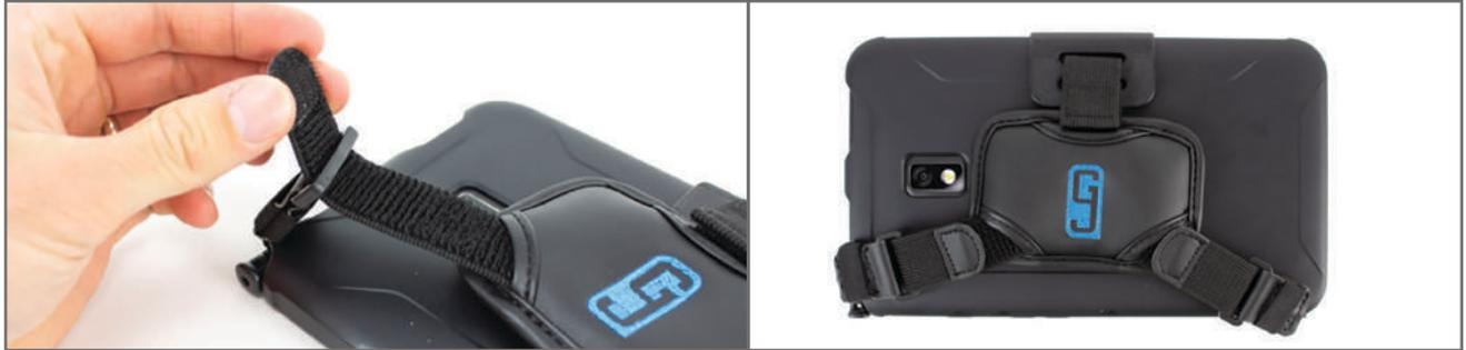
The Hand Pad Assembly (7) can now be secured to the Tab Active2. Start by feeding the Hook Velcro (5) ends through the two Buckle Loops (4) and the Plastic Retention Clip (8) in the positions shown above. Fold over the Hook Velcro and press it against the Loop Velcro (6) for a secure fit.
