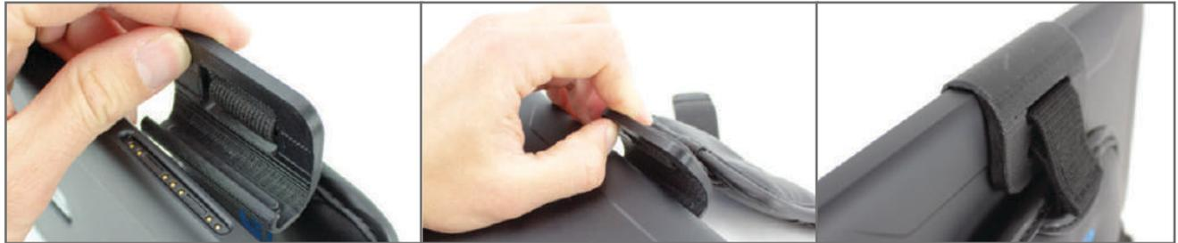
The Plastic Retention Clip (8) will be attached to the Tab Active2 where the outer case opens for the device charging pins. Hook the Clip (8) toward the Tab Active2 screen and press the clip down toward the back of the device. The Clip (8) may need to be adjusted slightly to match with the charging pin opening. If installed correctly, the Clip (8) will fit snug against the Tab Active2. Now your Y-Hand Strap is fully installed.
