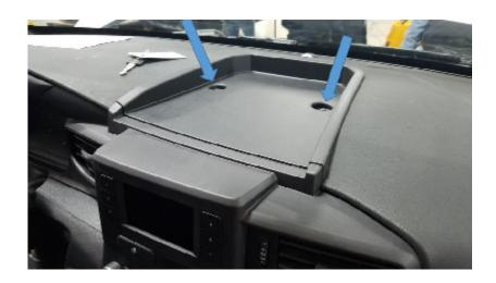
2. Place the GJ top tray inside the FORD OEM tray and reinstall with the OEM bolts.
