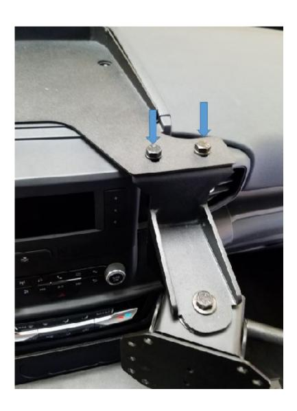
4. Attach the legs of the On-Dash to the top plate of the GJ Low-Profile Console as shown with 1/4 Allen head bolts provided, then attached the upper part of the legs to the vertical section of the On-Dash mount.
