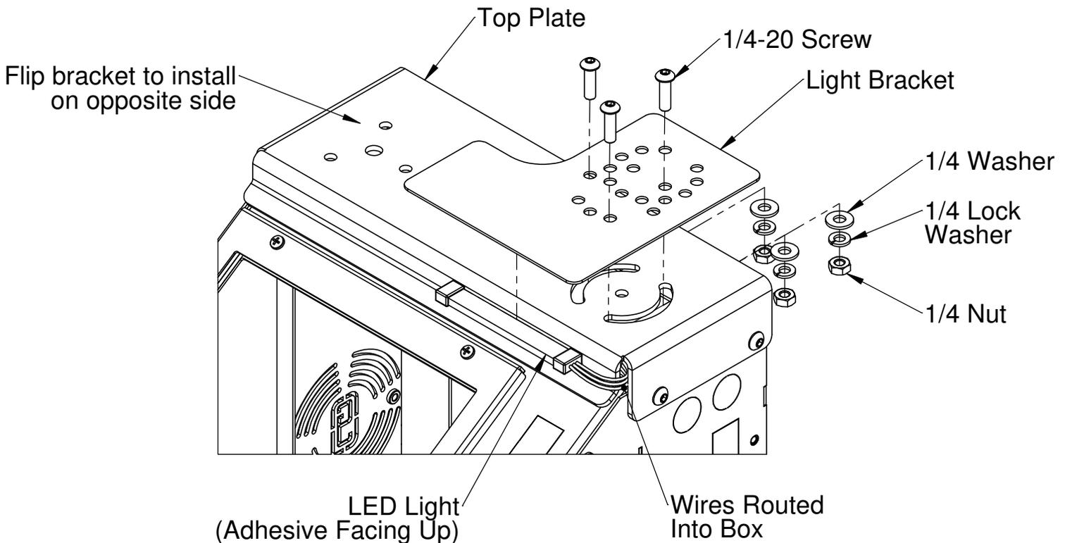
**FIG 1 - LED Light Bracket Installed**
