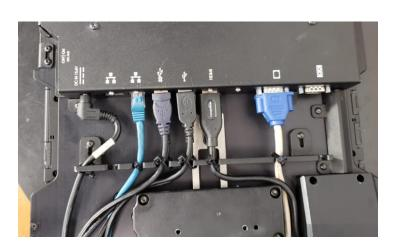
Connect all cables securely to dock ports, and use tie straps to secure cables to the "Cable Management Bar" as shown.
