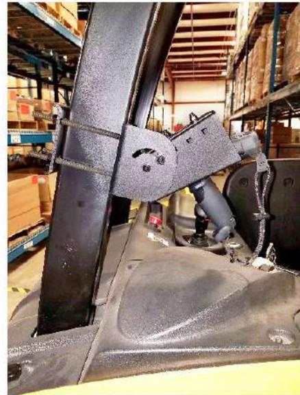
cap nuts to adjust width
