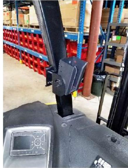
cap nuts to adjust width
