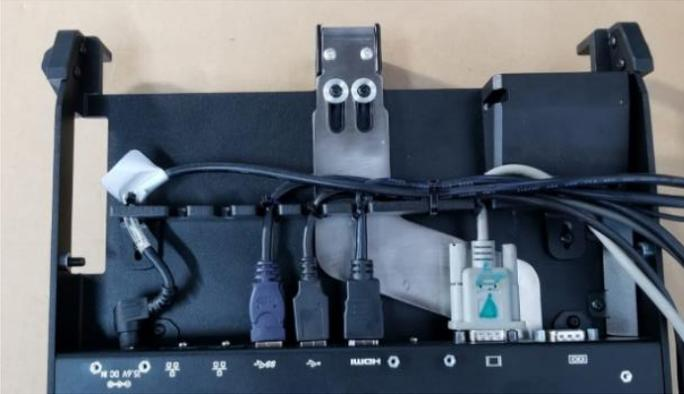
Connect all cables securely to dock ports, and use tie straps to secure cables to the “Cable Management Bar” as shown.
