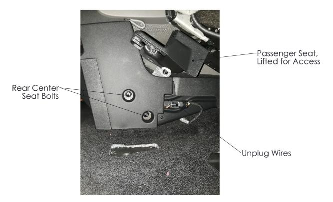
FIG 1 - Center Seat, Rear Passenger Side Bolts
