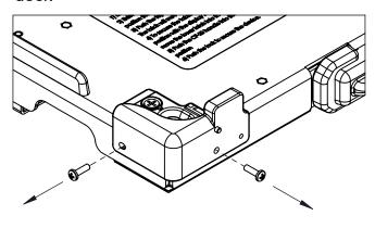
2 - Align the left tablet bracket and attach it to the dock with two of the screws included in the kit
