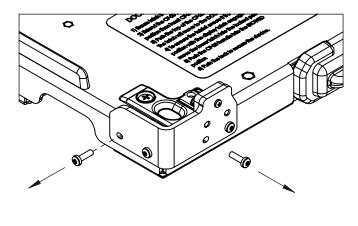
2 - Align the left tablet bracket and replace the two screws removed in step 1
