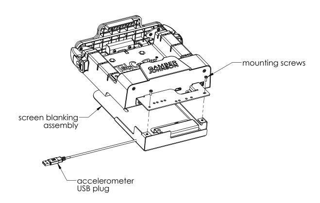
The dock (with the screen blanking assembly attached) can now be mounted using the mounting hardware typically supplied with the docking station.
