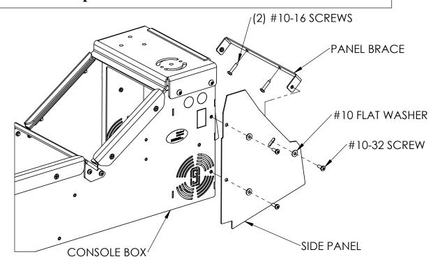
The side panels for the Ford Expedition (2007-2017) can be attached to the front of the console box to fill the gap between the console box and the vehicle's dash.
