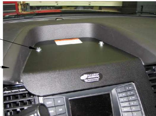
**Step 6. Attach the main bracket to the console box brackets installed in step 2 with two of the 1/4-20 x .50" long socket button head machine screws that were removed in step 1.**
