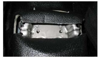
Fig 1 - Rear Mounting Bracket, Carpet Cut to Revel Threaded Inserts
