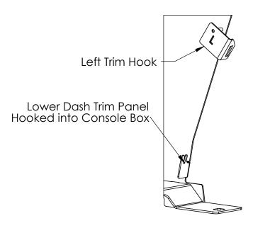
Fig 4 - Installing Lower Dash Trim Panels
