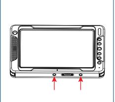
On the Bottom of the EX80 there are two holes. These holes are used to position and locate the EX80 into the dock.
