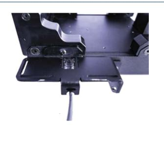
The cut out in the cable management bracket, allows the user to press the release clip on the RJ45 connector. This allow for easy tool free removal of the connector.
