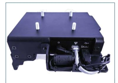
Connect all cables securely to dock connections. Use cable ties to secure cables to the built-in cable tie slots.
