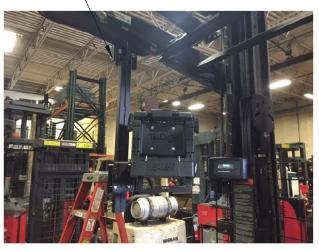
Views of pillar mount mounted on an Vertical Extension tube to position the computer equipment on the side of the fork truck
