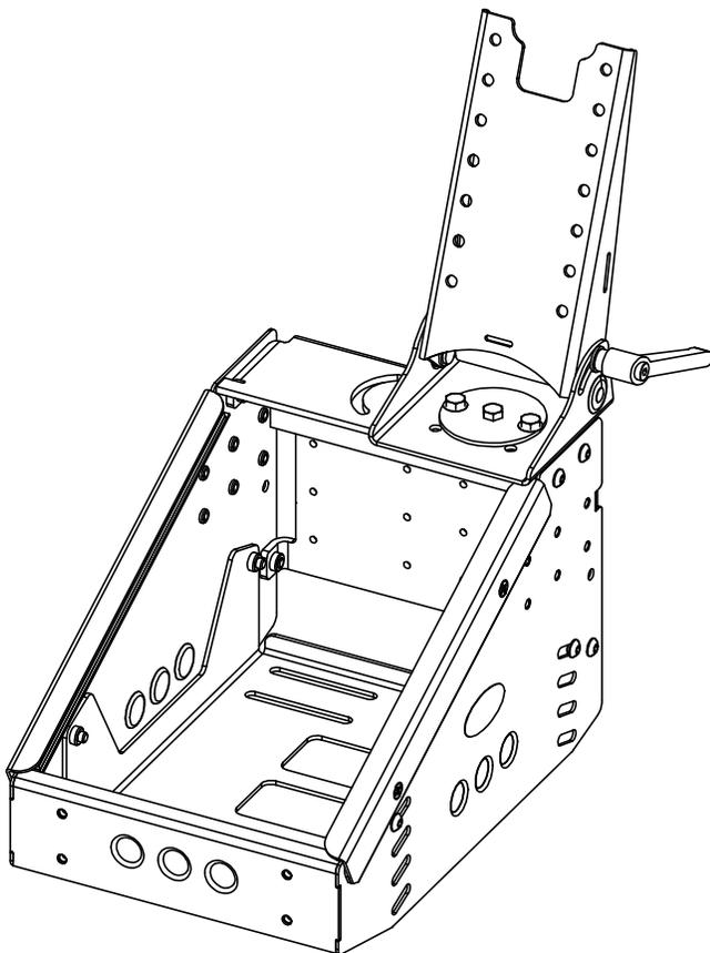
The Tablet Display Mount can be mounted on any Gamber-Johnson pole or console with a swivel pattern cutout or 3/8" mounting hole.
