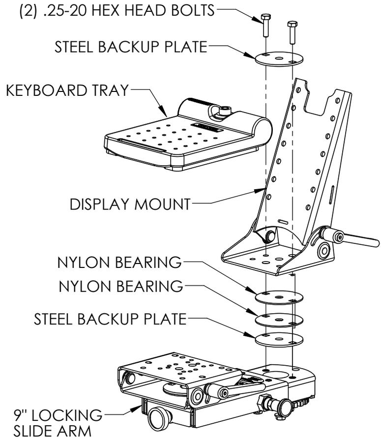
The Tablet Display Mount can also be mounted on various Gamber-Johnson Motion Attachments, which are then mounted on a console or pole.
