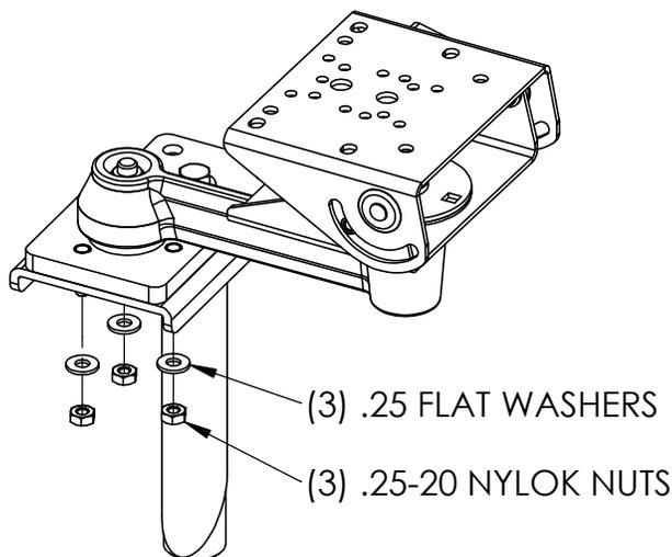
Remove the .25-20 nylok nuts and flat washers from the adapter plate. Place the adapter base on the upper pole assembly, inserting the threaded studs through the two radial slots. Place the washers and lock nuts on the studs and tighten. Unscrew the tilt knob to loosen clevis assembly and set the amount of tilt. Lock in place by tightening knob.
