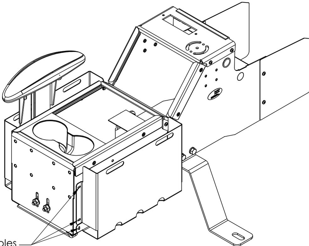
Drill 3/16" dia. holes at these locations on each side of the pocket
