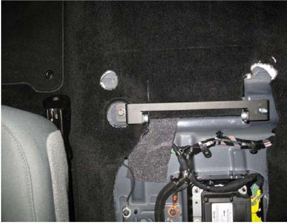
3. Attach Front Leg to center seat section mounting point, reusing original seat bolt or the M8 bolt supplied in the hardware bag.
