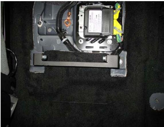
5. Attach Rear Leg to center seat section mounting points, reusing original seat bolts or the M8 bolts supplied in hardware bag.
