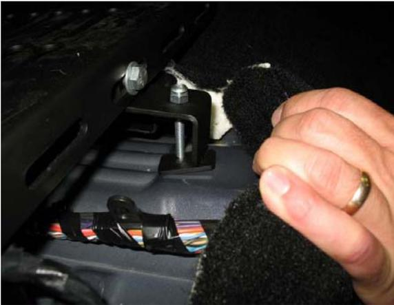
4. Tighten the 1/4-20 x 2.00 Socket Button Head Screw with a 5/32" Hex bit against Clamp Plate, until the Front Leg Tab is wedged in mounting hole.
