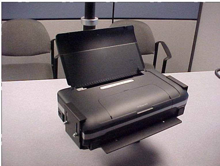
4. Insert printer into printer mount. Center printer so paper feed doors can be opened. Move side and back brackets against printer body and tighten in place. Attach and secure power and data transfer cables.
