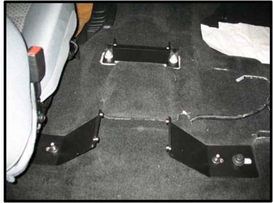
6. Install the Top Plate using (6) .38-16 bolts and washers supplied in hardware bag. Adjust Back Legs so Top Plate is aligned with center of vehicle. Tighten all nuts and drivers side seat bolts. Reinstall trim pieces on rear drivers seat brackets.
