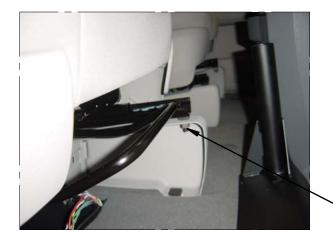
Move the front passenger seat rearward to gain access to the front inboard and outboard bolts. Remove the nuts from the bolts. Place an open ended wrench between the seatrail and seatbase onto the iam nut. Unscrew bolts using torx bit until you are able to lift seat enough to slide item 7160-0116 between the seatrail and seatbase. Retighten bolts back down and replace the nuts.
