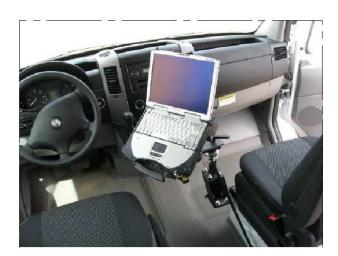
Complete the install by attaching upper pole, motion attachment and dock or cradle assemblies as required.
