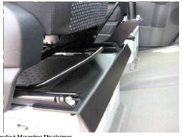
Insert Sprinter base between seatrails and seat
