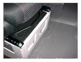
Move passenger seat forward to gain access to two seatbolts which attach the seattrails to the back of the seat base.
