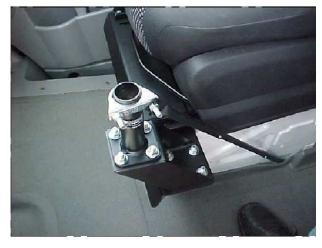
A LAC-03 support base is strongly recommended for extra stability. Attach LAC-03 support brace between lower tube assembly and seat base.
