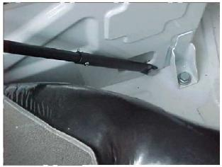
On 2007 and newer vehicles an existing hole in the seat base can be used as a mounting point.
